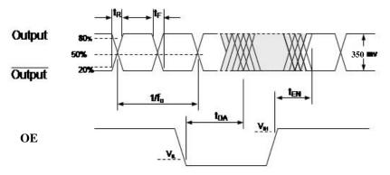
Figure 2. LVDS Output Waveform
