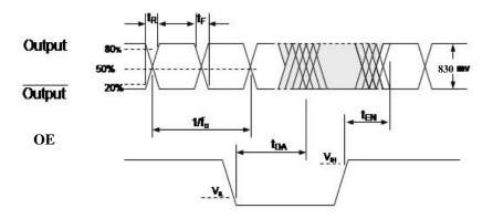
Figure 3. LVPECL Output Waveform
