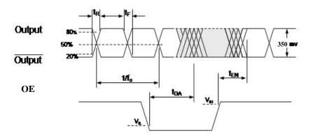
Figure 4. LVDS Output Waveform
