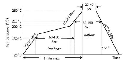
Figure 5. Solder Reflow Profile
