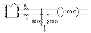
$R_{\text{S}}$  is a series resistor implemented to match the trace impedance. Depending on the board layout, the value may range from 0 to 30Ohms
