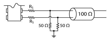
$R_{\text{S}}$  is a series resistor implemented to match the trace impedance. Depending on the board layout, the value may range from 0 to 30Ohms
